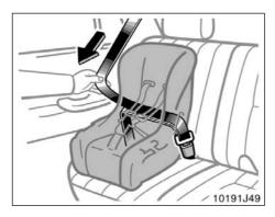
Fully extend the shoulder belt to put it in the lock mode. When the belt is then retracted slightly, it cannot be extended.
