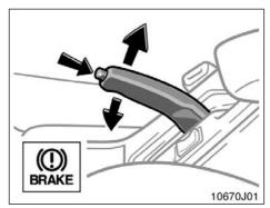
When parking, firmly apply the parking brake to avoid inadvertent creeping.
