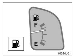
The gauge works when the ignition switch is on and indicates the approximate quantity of fuel remaining in the tank.
