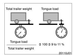
● The trailer cargo load should be distributed so that the tongue load is 9 to 11% of the total trailer weight, not exceeding the maximum of the following. Never load the trailer with more weight in the back than in the front. About 60% of the trailer load should be in the front half of the trailer and the remaining 40% in the rear.
