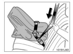
Fully extend the shoulder belt to put it in the lock mode. When the belt is then retracted even slightly, it cannot be extended.
