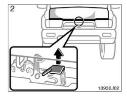
In front of the vehicle, pull up on the auxilialy catch lever and lift the hood.
