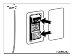
LOCKING AND UNLOCKING WITH POWER BACK DOOR LOCK SWITCH
