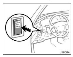
Never use the switch for normal engine starting. Be sure to follow the starting procedure instructed in "How to start the engine" in Part 3.
