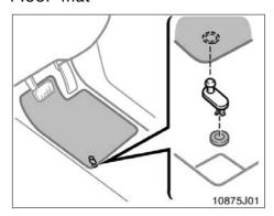
Use a floor mat of the correct size. If the floor mat has a hole, then it is designed for use with a locking clip. Fix the floor mat and locking clip into the hole in the floor carpet.
