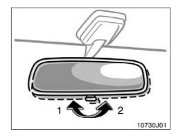
To reduce glare from the headlights of the vehicle behind you during night driving, operate the lever on the lower edge of the mirror.
