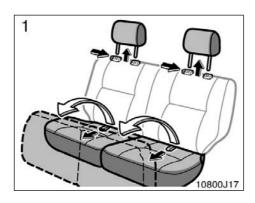
Remove the head restraint, and swing the bottom cushion up by pulling the lock release strap. Be certain to replace the head restraint.
