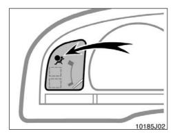
This SRS airbag system has a service reminder indicator to inform the driver of operating problems. If either of the following conditions occurs, this indicates a malfunction of the airbags. Contact your Toyota dealer as soon as possible to service the vehicle.
