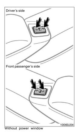
LOCKING AND UNLOCKING WITH POWER DOOR LOCK SWITCH
