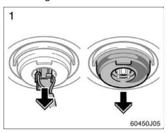
Open the hood. Unplug the connector. Remove the rubber cover.
